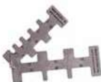
Bead gauges for checking final bead width (see p24)
