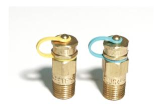
Pete's Plug II is available in various pipe thread sizes, lengths and materials to satisfy each application. The XL Pete's Plug II will allow you to insulate the test point and not completely cover the Pete's Plug II. The XL Pete's Plug II eliminates extra fittings for insulated applications.
